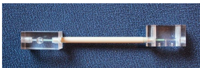
Figure 14: Long path length uv-vis Garth cell
